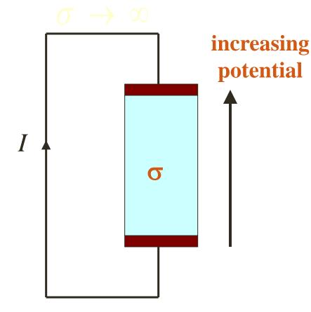
The current / must be zero since the electrons cannot gain back the energy they lose in traveling through the resistor.
