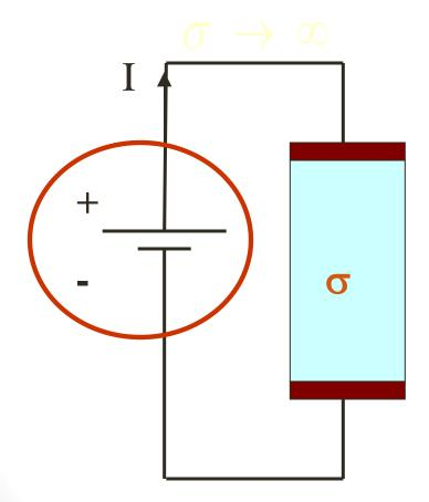
To maintain a steady current, there must be an element in the circuit wherein the potential rises along the direction of the current.
